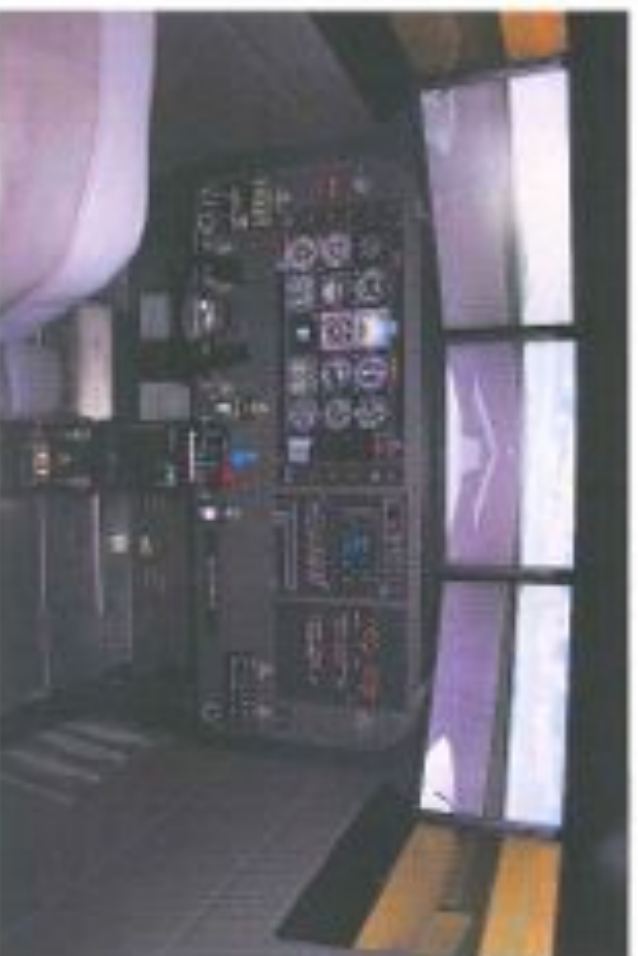
Figure 1 DCX™ cockpit system with integrated 225-degree 5-channel visual system.
